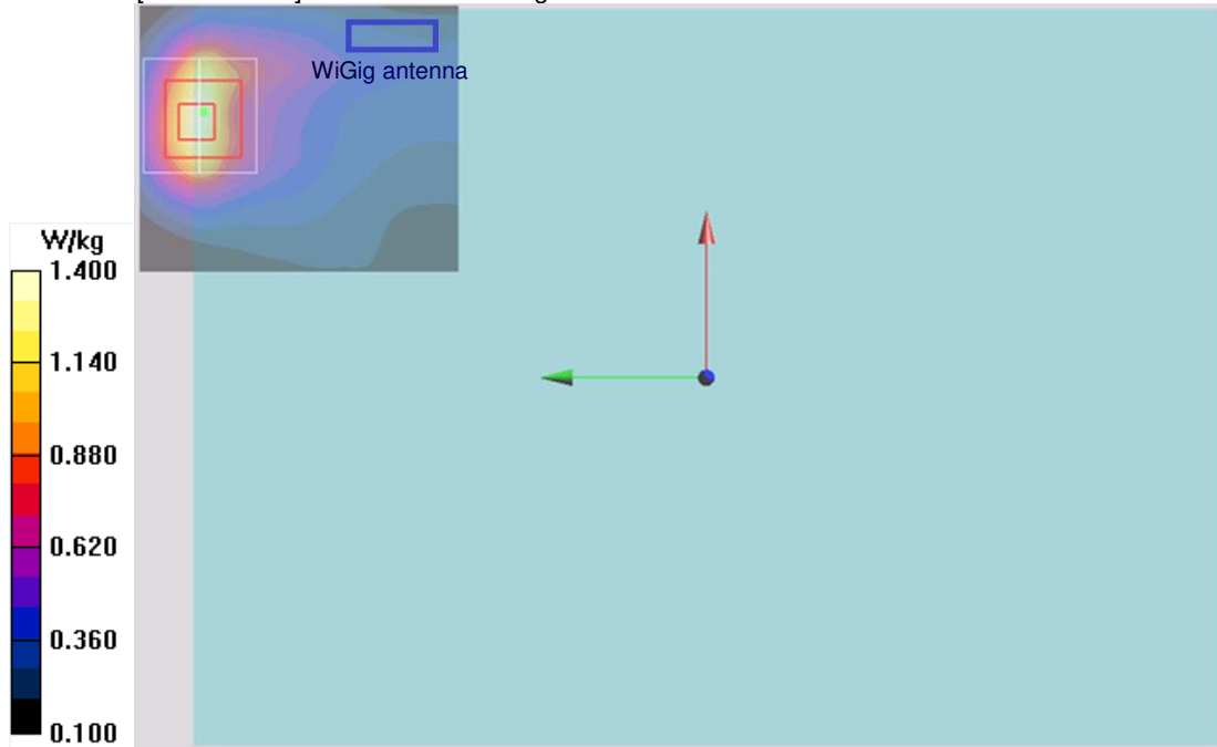
[Bottom Face] WWAN with WiGig at 11mm
