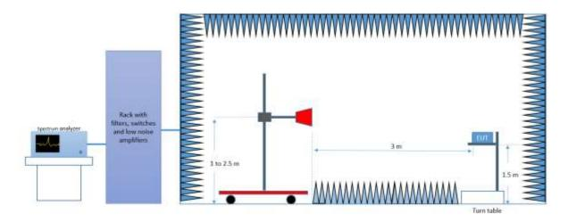
Radiated Setup 18 GHz - 26.5 GHz
