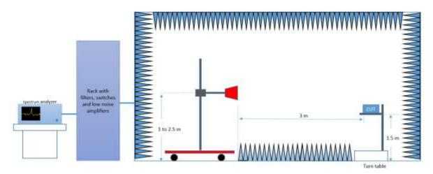
Radiated Setup 18 GHz - 26.5 GHz
