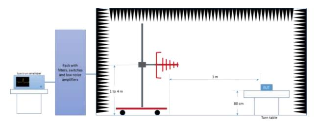
Radiated Setup 1 GHz - 18 GHz
