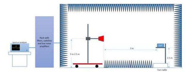
Radiated Setup 18 GHz - 26.5 GHz
