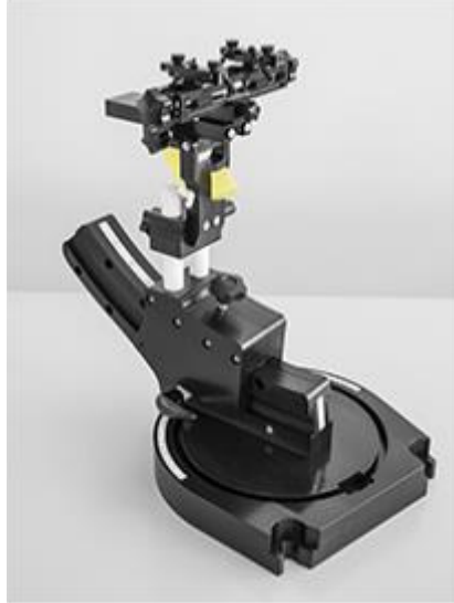
Mounting Device for Hand-Held Transmitters
