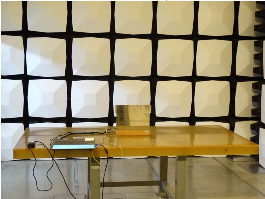
Back View of Radiated Test (Horn)
