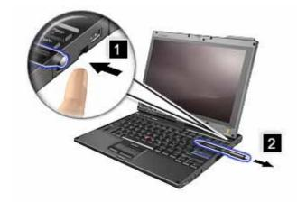
**Note:** The pen contains pressure sensors. Do not push the tip of the pen for an extended period of time. Do not subject the pen to shock or vibration.
