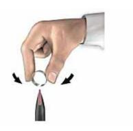
2. Insert a replacement pen tip fully into the Tablet Digitizer Pen.
