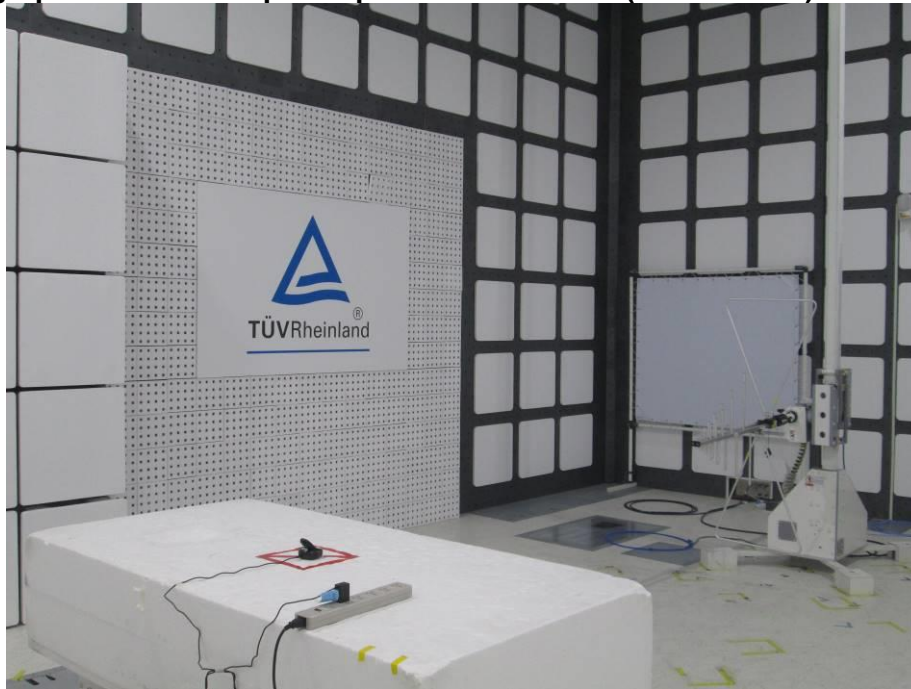
Photograph 21: Test Setup for Spurious Emissions (Back View 2)
