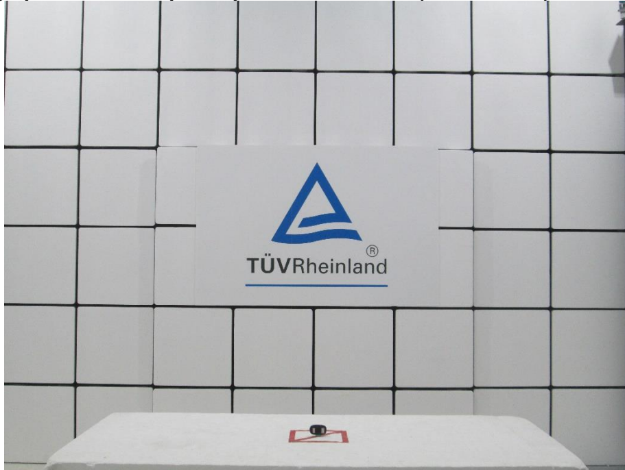
Photograph 8: Test Setup for Spurious Emissions (Front View 2)
