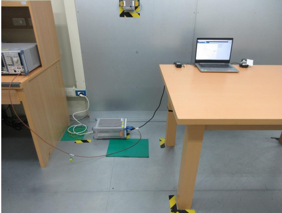
Photograph 22: Test Setup for Mains Conducted Emissions (Front View)
