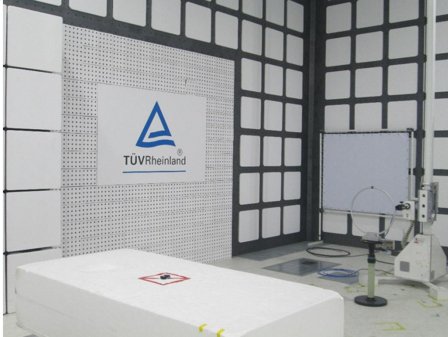
Photograph 3: Test Setup for Spurious Emissions (Back View 1)
