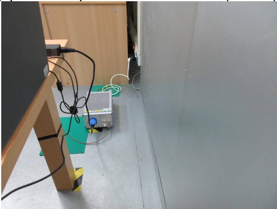
Photograph 23: Test Setup for Mains Conducted Emissions (Back View)
