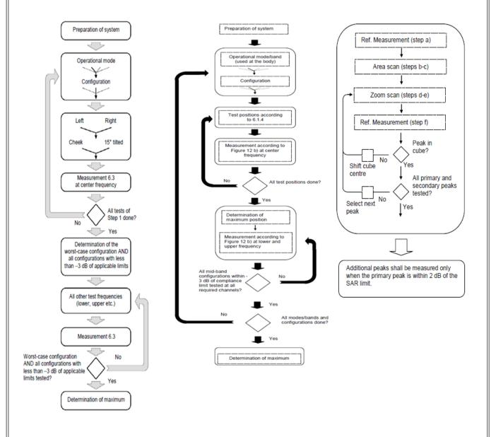
After an area scan has been done at a fixed distance of 1.4mm from the surface of the phantom on the source side, a 3D scan is set up around the location of the maximum spot SAR. First, a point within the scan area is visited by the probe and a SAR reading taken at the start of testing. At the end of testing, the probe is returned to the same point and a second reading is taken. Comparison between these start and end readings enables the power drift during measurement to be assessed.
