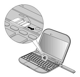
4. Insert the SIM card into the slot, as shown in the figure below, and press it firmly until it stops.
