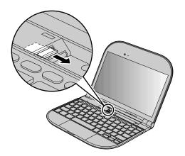
Insert a card into the slot, as shown in the figure below, and press it firmly until it stops.
