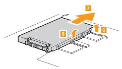
8 Take out the hard disk drive secured in the hard disk drive bay.
