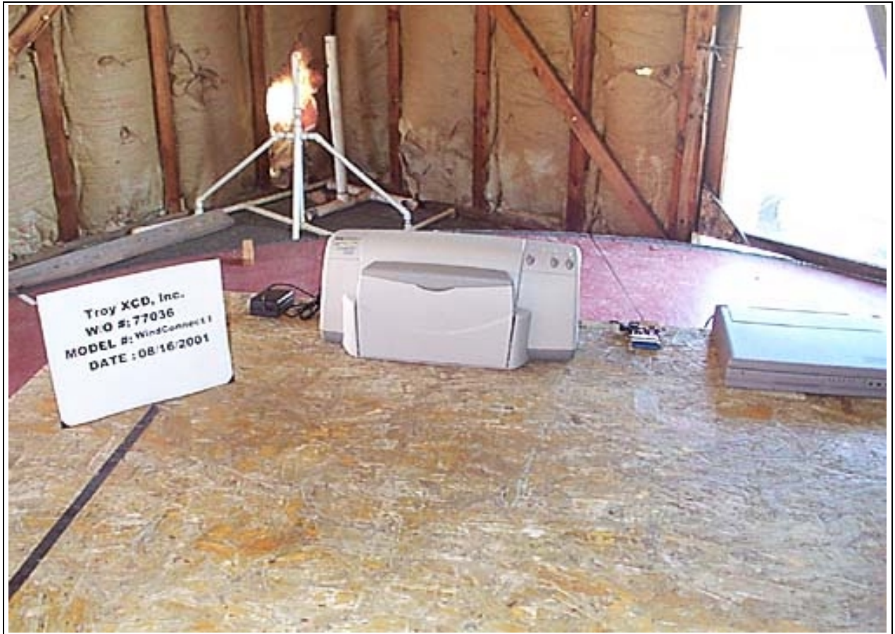
Radiated Emissions - Front View (Mariposa Setup)
