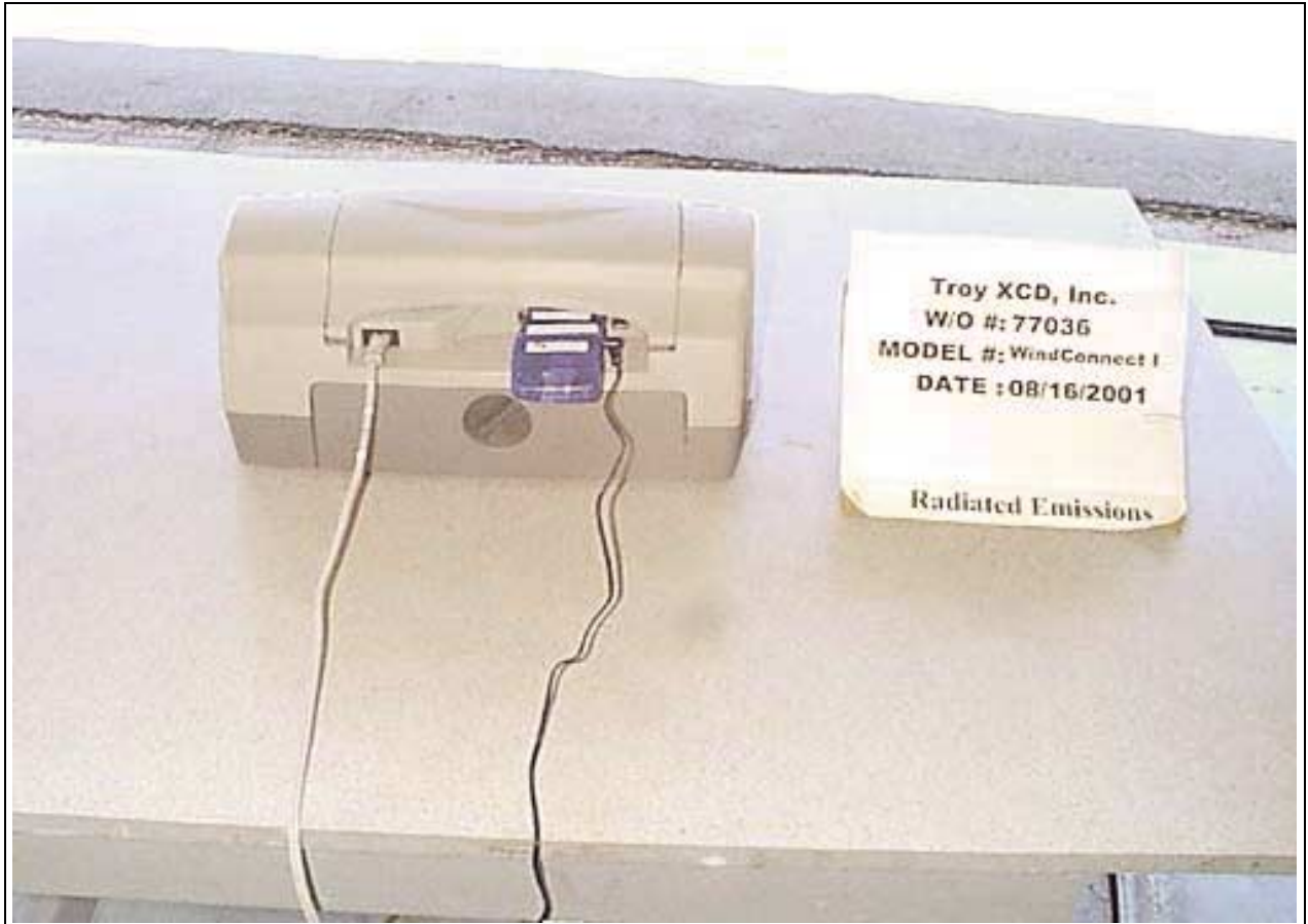
Radiated Emissions - Back View (Brea Setup)
