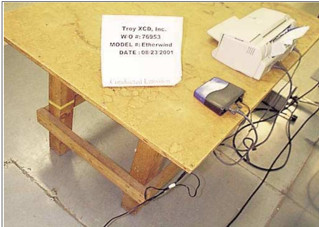
Conducted Emissions - Back View
