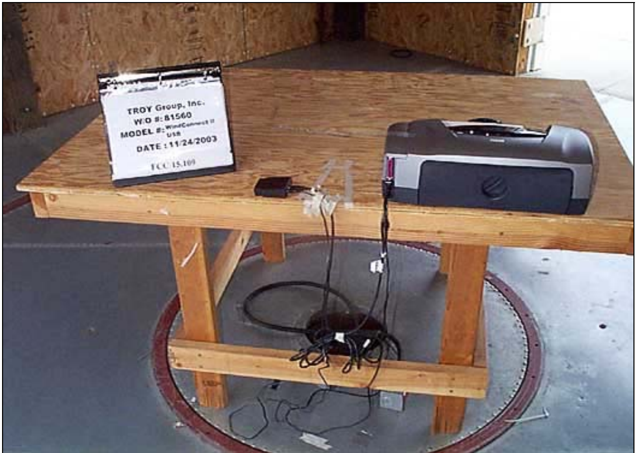
11/24/03 Radiated Emissions - Back View USB
