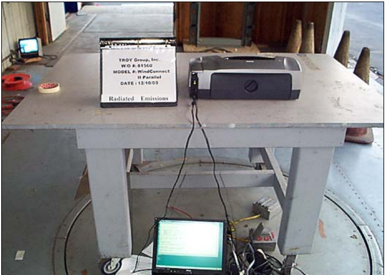
12/10/03 Radiated Emissions - Back View Parallel
