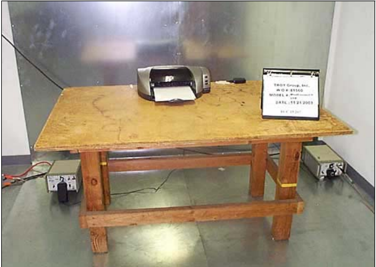
Mains Conducted Emissions - Front View USB
