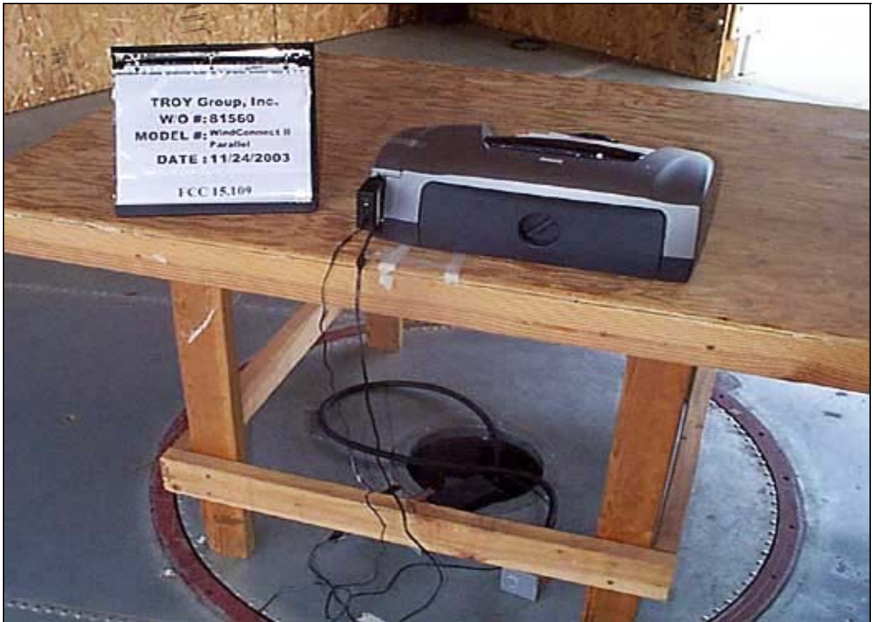
11/24/03 Radiated Emissions - Back View Parallel
