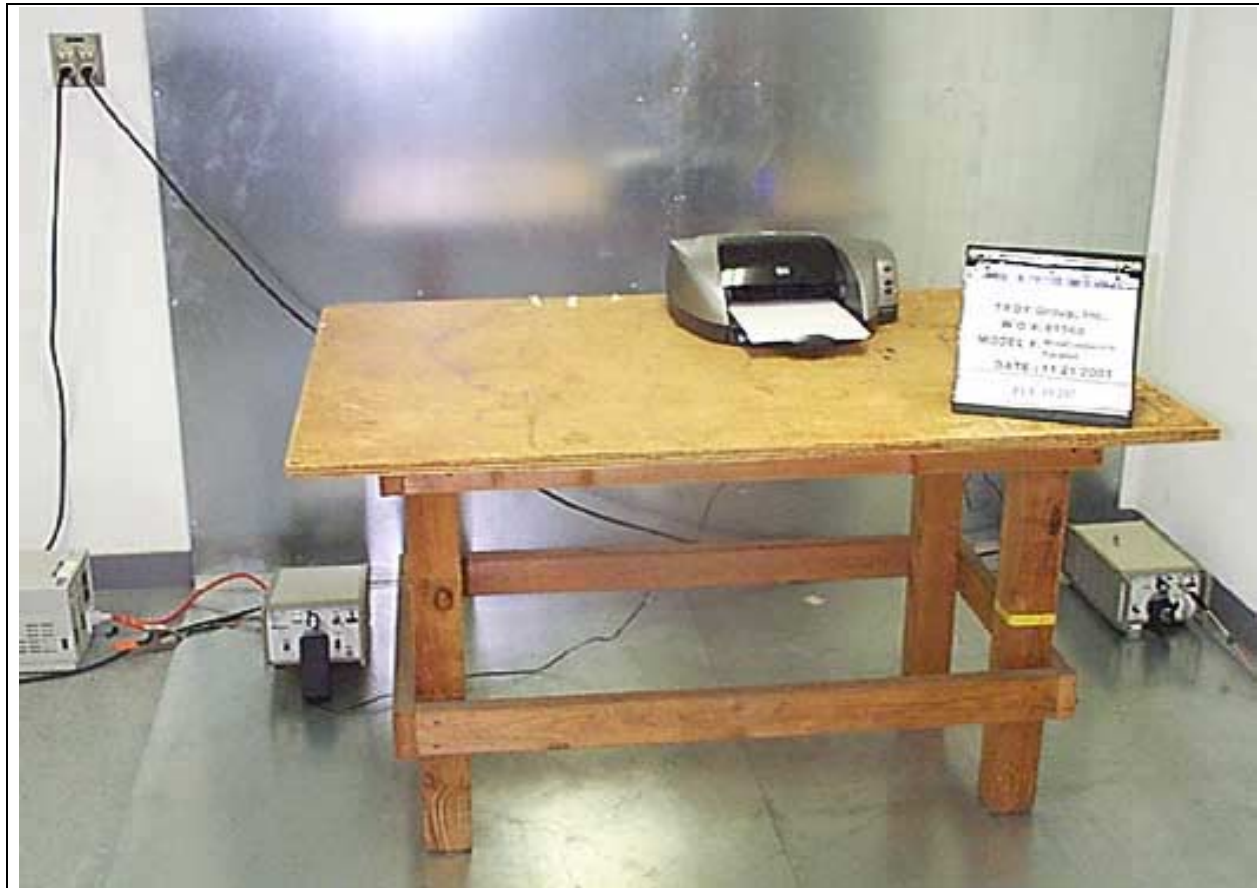
Mains Conducted Emissions - Front View Parallel
