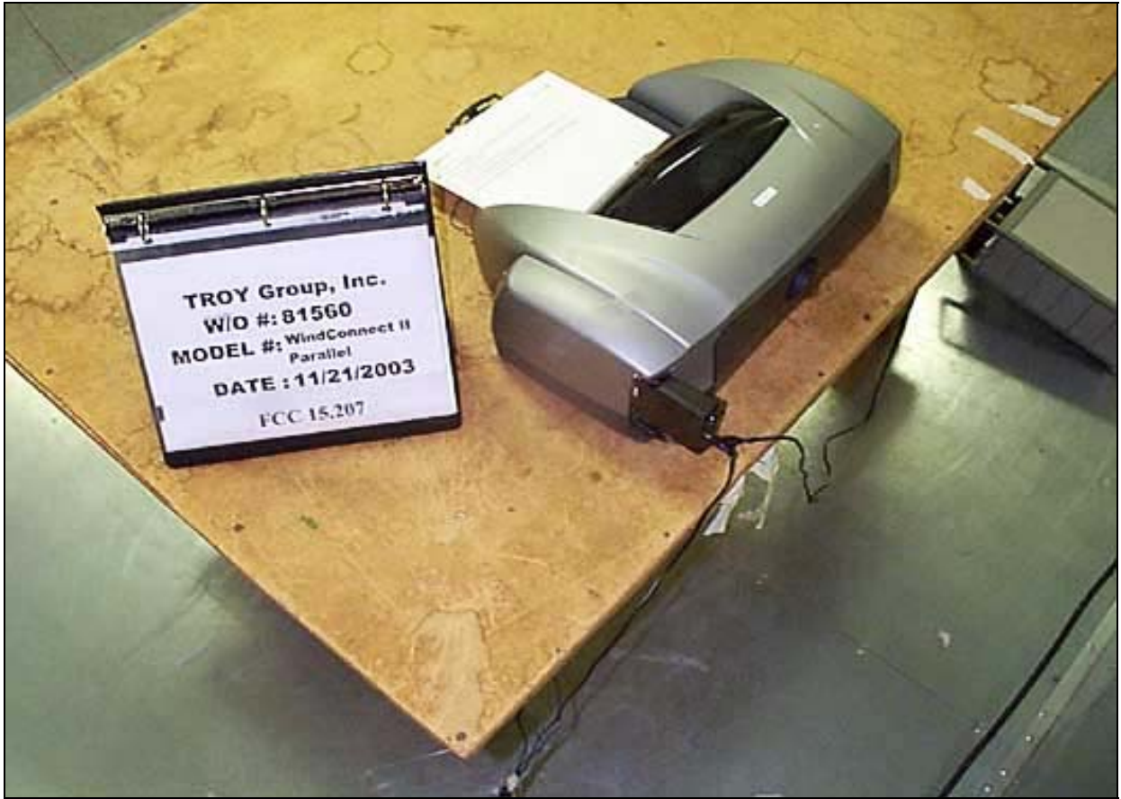
Mains Conducted Emissions - Back View Parallel
