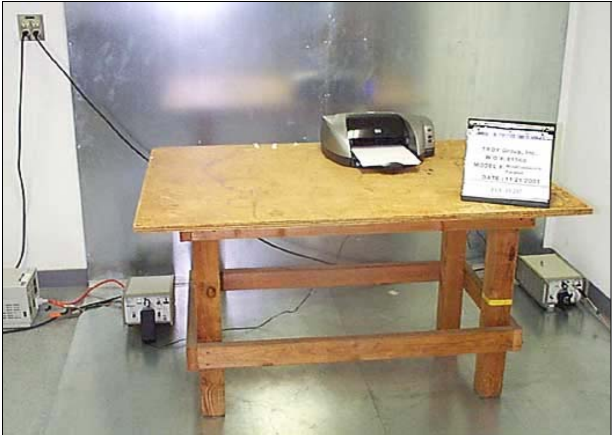
Mains Conducted Emissions - Front View Parallel
