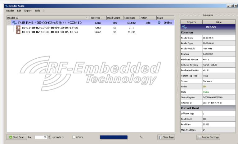
Now you can start an inventory with the just added reader using the “Start Scan” button at the bottom left of the application. If a tag is detected, it is shown in the tree view below the reader:
