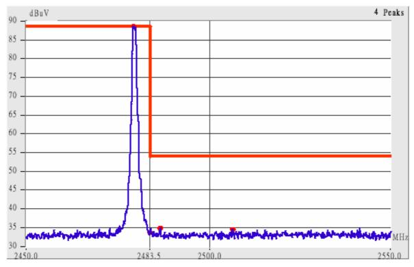
This is the hard copy of our bandedge measurement generated by our bandedge testing program. The plot shown above is the bandedge of channel 78.
