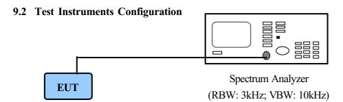
PC to control the EUT at maximal power output and channel number and set antenna kit
