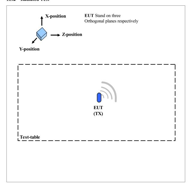
The tests below are carried with the EUT transmitter set at high power in TDD mode. The EUT is forced to select of output power level and channel number by notebook computer.
