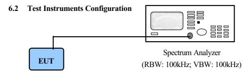
EUT set testing mode, Press function keys of EUT to control the EUT at maximal power output and channel number
