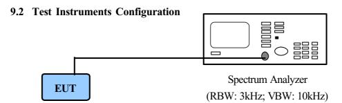
EUT set testing mode, Press function keys of EUT to control the EUT at maximal power output and channel number
