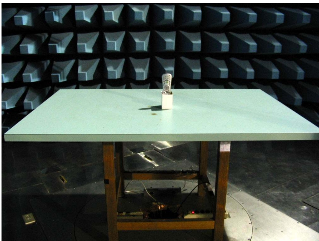
The Test Configuration of Y-plane
