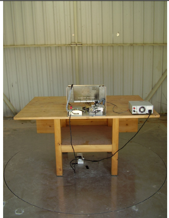
RE test setup on OATS
