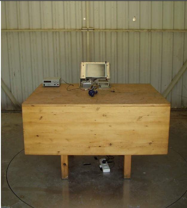
RE test setup on OATS
