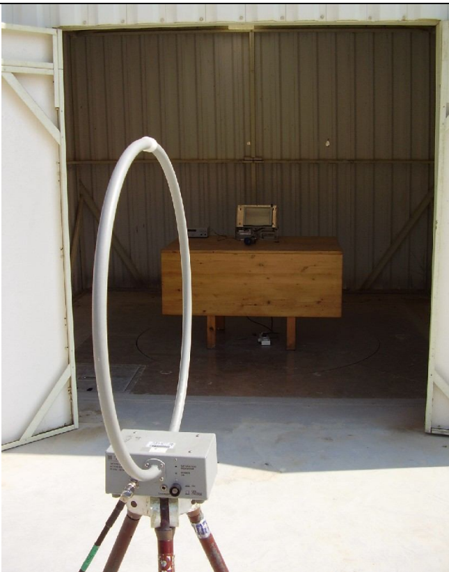
RE test setup on OATS (below 1 GHz)
