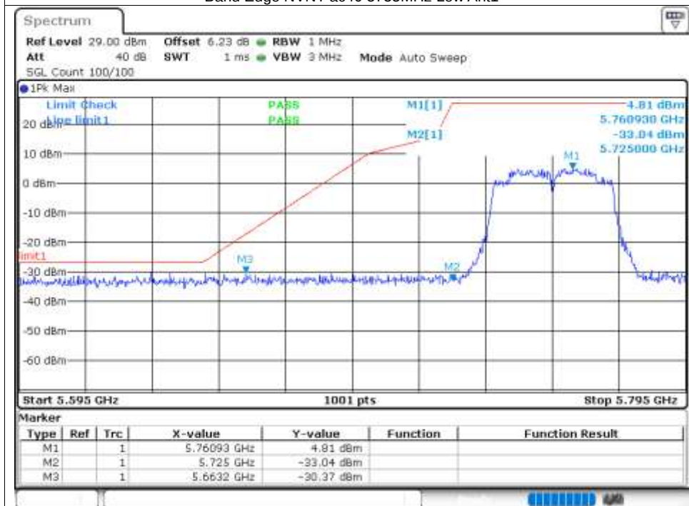
Band Edge NVNT ac40 5795MHz High Ant1
