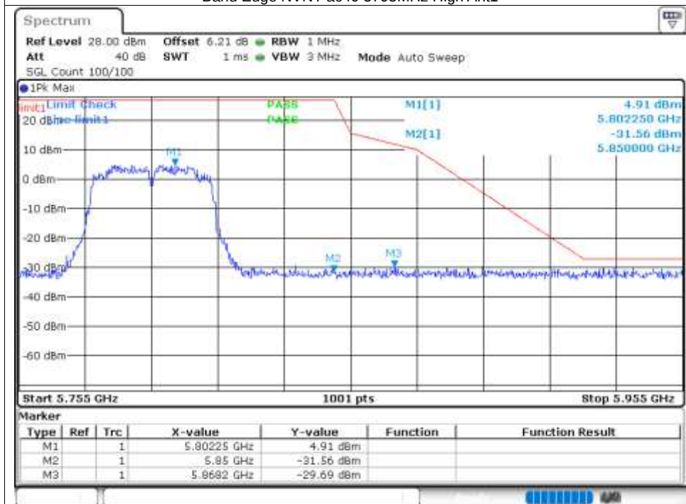
Band Edge NVNT ac40 5795MHz High Ant1
