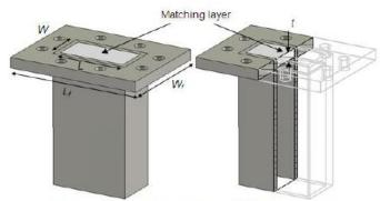
Figure 1: Validation Waveguide Dimensions
