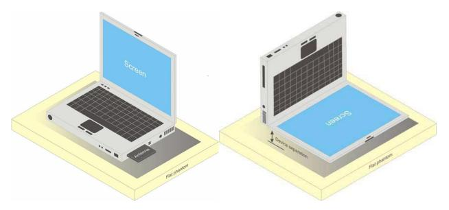
Figure 6.1 – Test positions for Laptop
