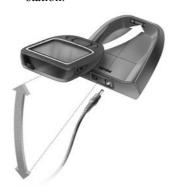
Charging starts immediately. The blue charging LEDs on the front of the docking station indicate that the battery pack is being charged.
