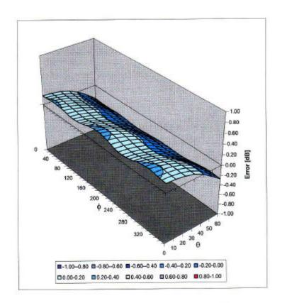
Spherical Isotropy Error < ± 0.4 dB
