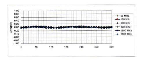
Axial Isotropy Error < ± 0.2 dB
