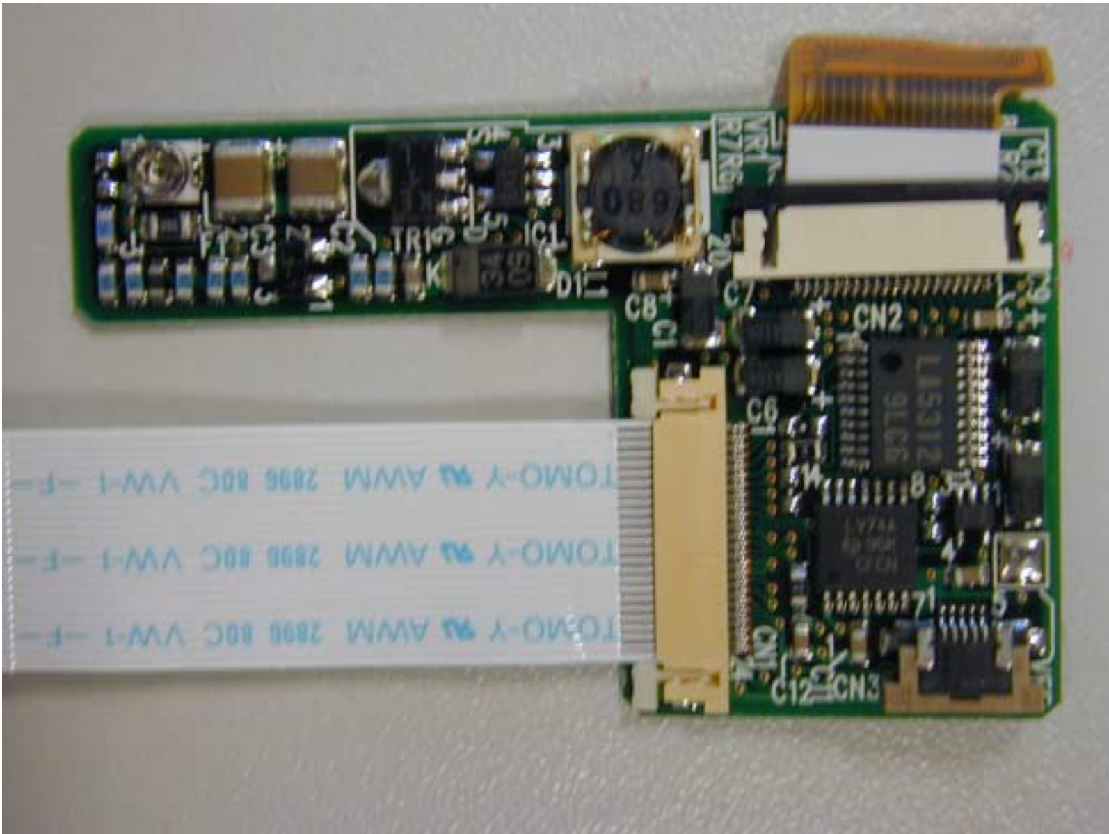
CONTROLLER BOARD TOP
