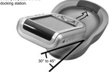
Charging starts immediately. The blue charging LED on the front of the docking station indicates charging takes place. When the RC5400 is fully charged, the LED goes off.
