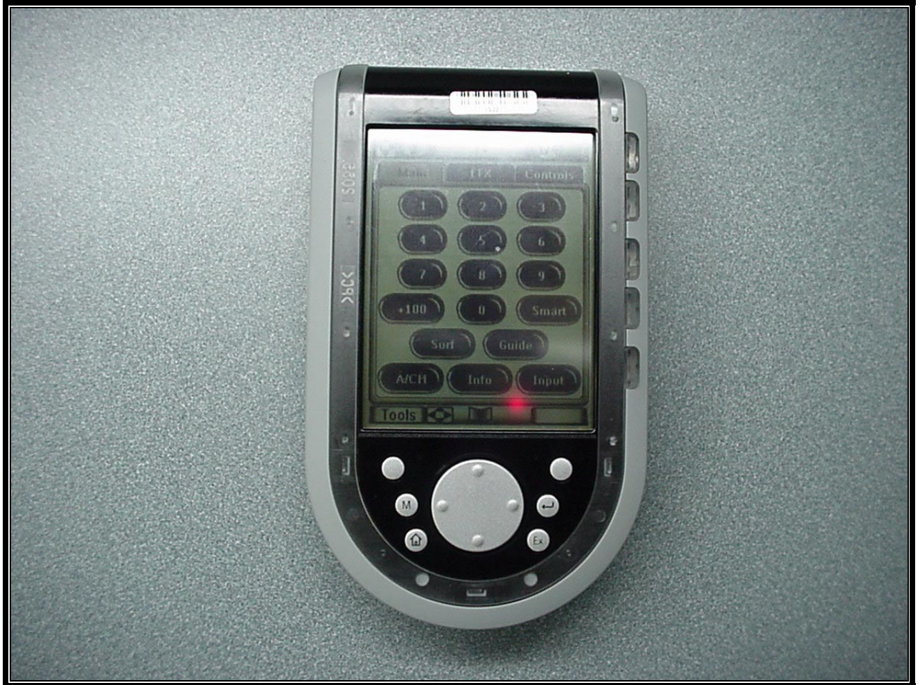
PHOTOGRAPH 8: FRONT VIEW OF TOUCH SCREEN REMOTE CONTROL
