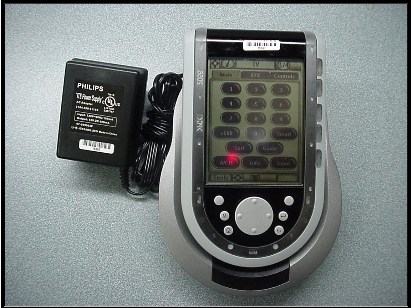
PHOTOGRAPH 7: TOUCH SCREEN REMOTE CONTROL IN DOCKING STATION
