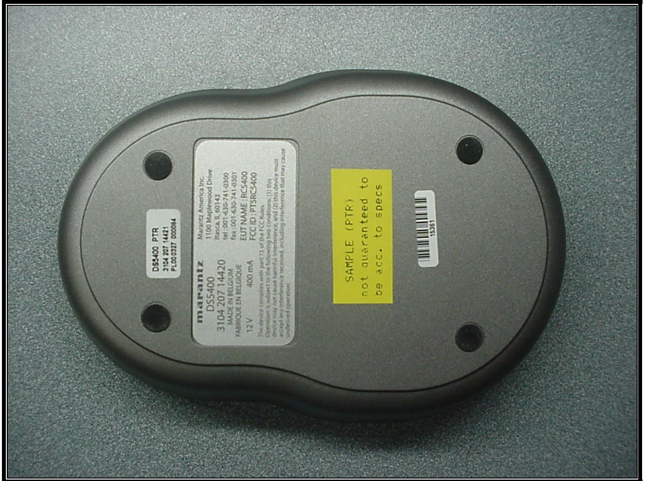
PHOTOGRAPH 15: BOTTOM VIEW OF DOCKING STATION
