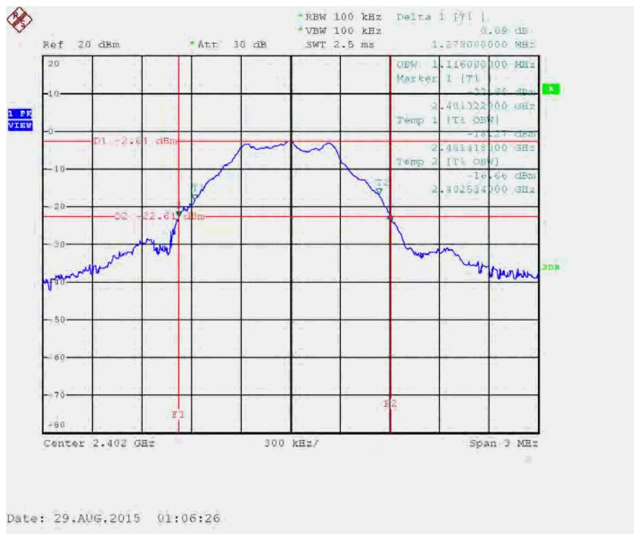
**20 dB/99% Bandwidth Plot on 2442 MHz**
