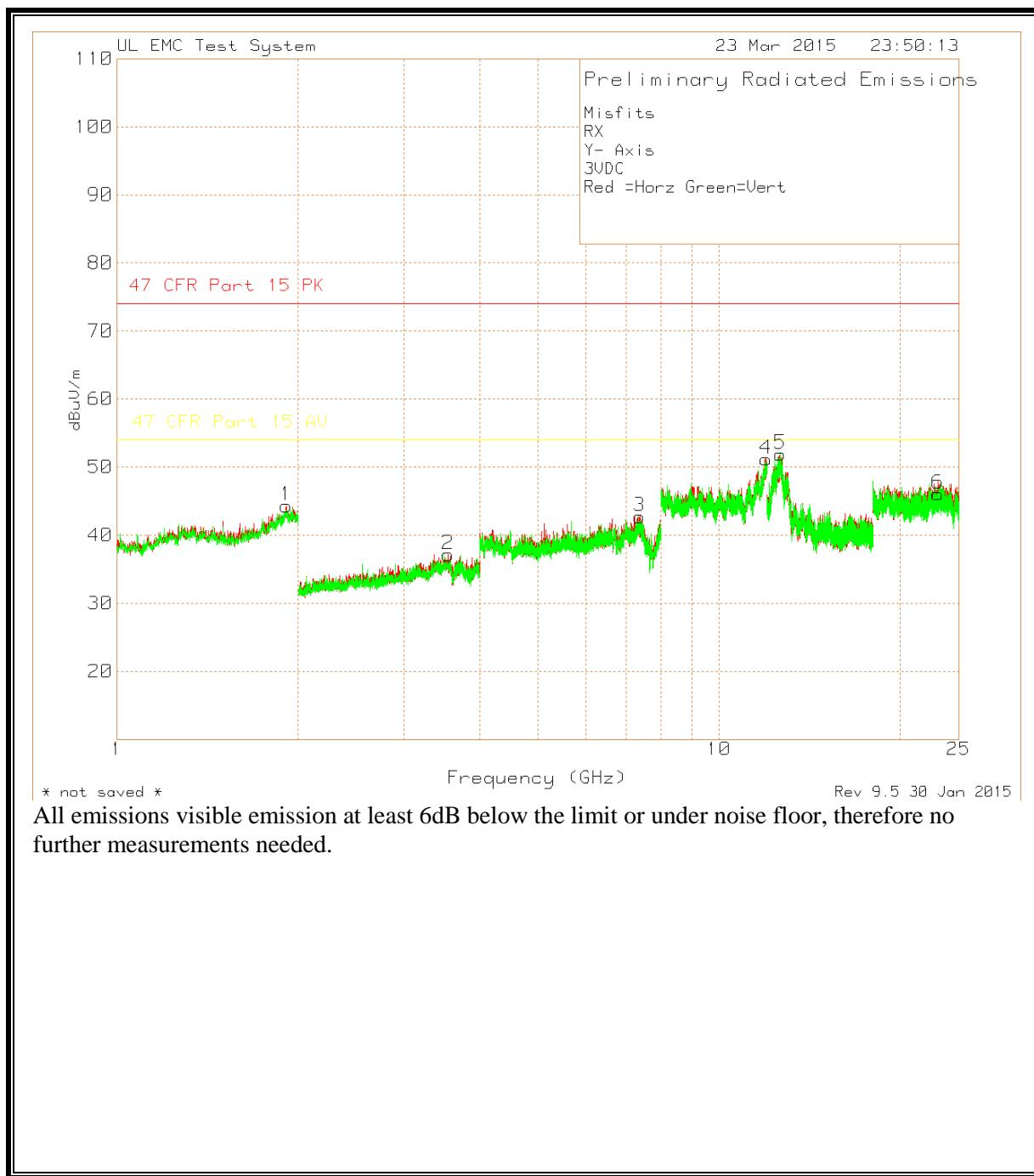
All emissions visible emission at least 6dB below the limit or under noise floor, therefore no further measurements needed.
