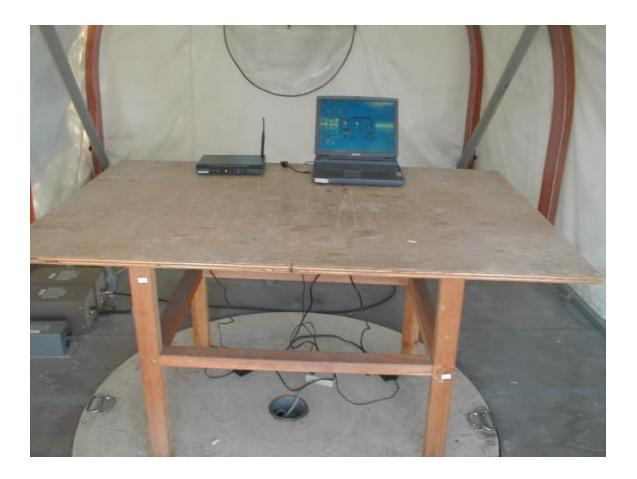
Radiated Emission Setup Photograph – Rear View
