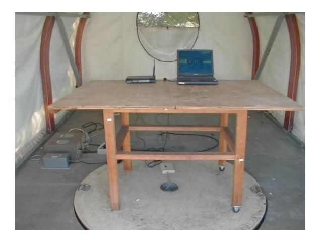
Conducted Emission Setup Photograph -Rear View
