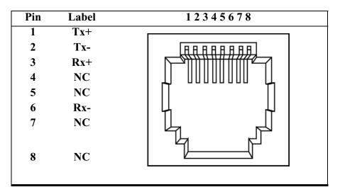
Figure B.1 10/100 Ethernet Port Pinout
