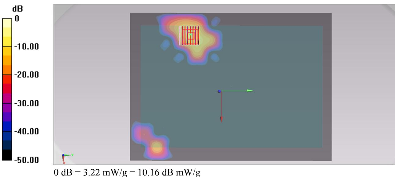
**#17 WLAN5G\_802.11a\_Bottom Face\_0cm\_Ch165\_2D****DUT: 283001**
