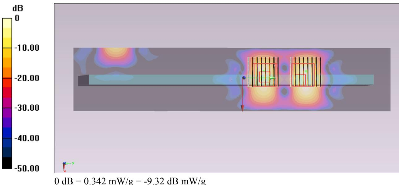
**#08 WLAN5G\_802.11a\_Edge3\_0cm\_Ch36\_2D****DUT: 283001**
