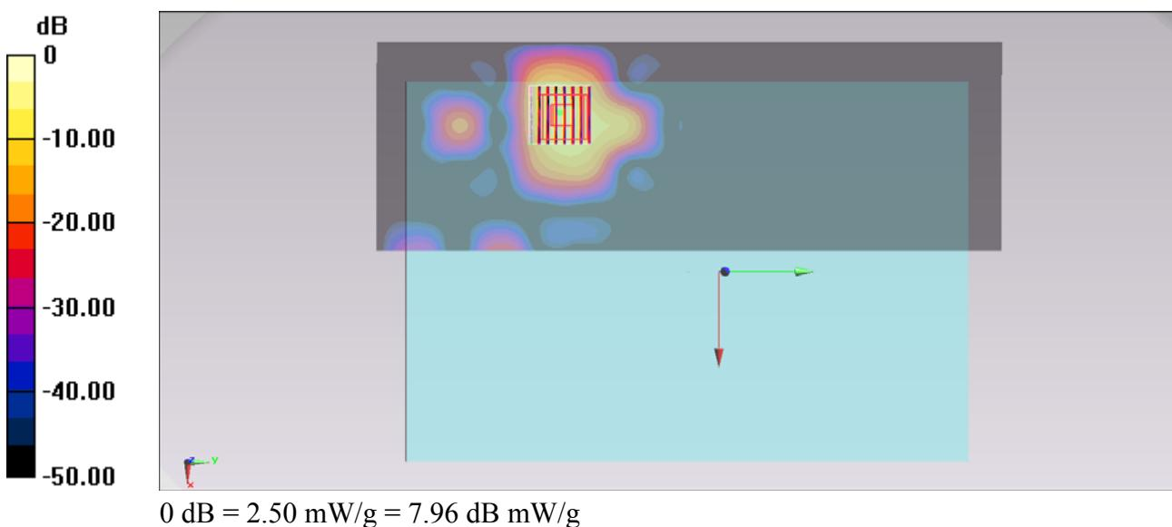
**#19 WLAN5G\_802.11a\_Bottom Face\_0cm\_Ch157****DUT: 283001**
