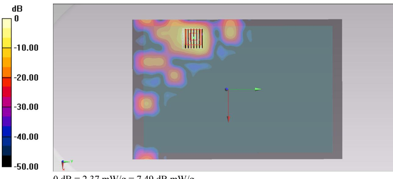
**#14 WLAN5G\_802.11a\_Bottom Face \_0cm\_Ch108****DUT: 283001**
