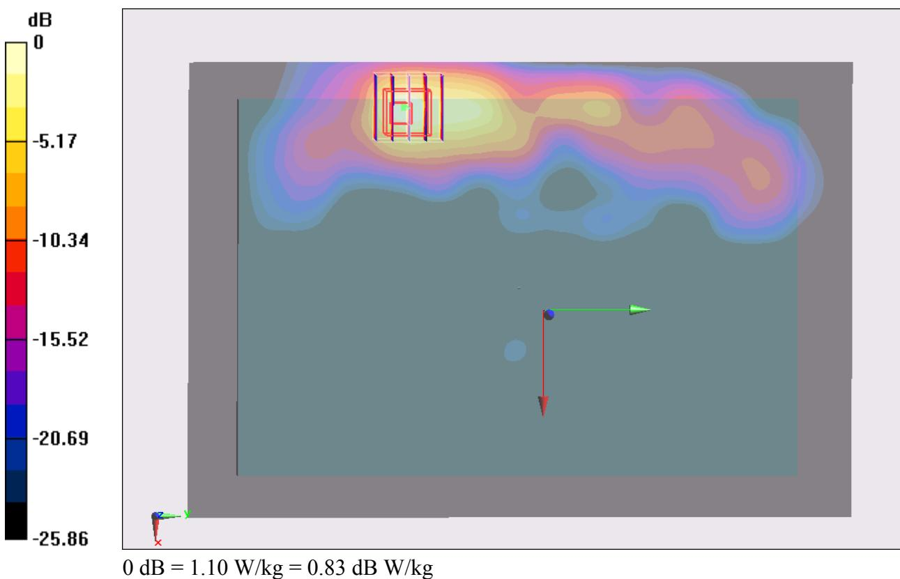
**#03 WLAN2.4G\_802.11b\_Bottom Face\_0cm\_Ch11\_2D****DUT: 283001**
