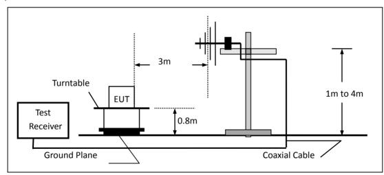
(c) For radiated emissions above 1000MHz
