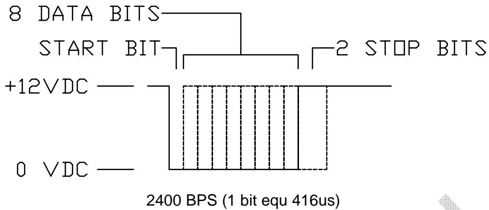
The control string is transmitted as seven (7) bytes, 2400 bps, 8 data bits, 2 stop bits. The function of each byte is as follows:
