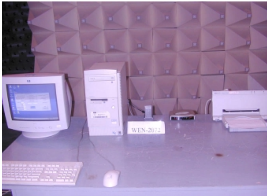
Photo 2: Radiated Emission Test Set-up (rear)
