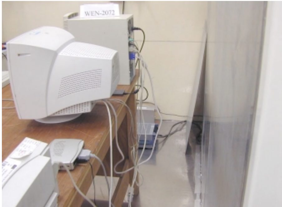
Photo 2: Conducted Test Set-up (rear)
