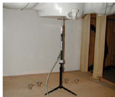
Figure 12.1 Dipole Validation Test Setup
