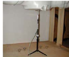
Figure 9.1 Dipole Verification Test Setup Diagram & Photo
