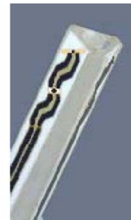
Figure 3.3 Probe Thick-Film Technique
