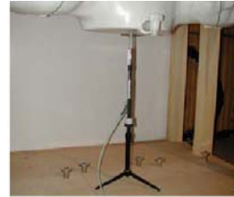
Figure 9.1 Dipole Verification Test Setup Diagram & Photo
