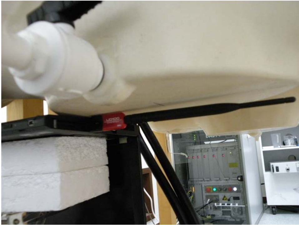
<Vertical & Ant Horizontal R-AN2400-1901RS (19.7 cm)>
