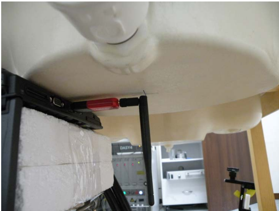
<Horizontal Up & Ant Vertical_R-AN2400-5801RS(13.7cm)>
