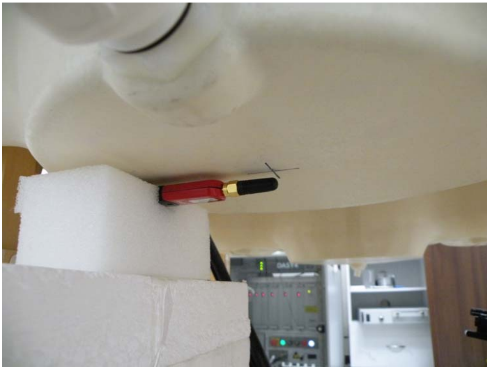
<Horizontal Down & Ant-Fixed_AN2400-3306RS(3.0cm)>
