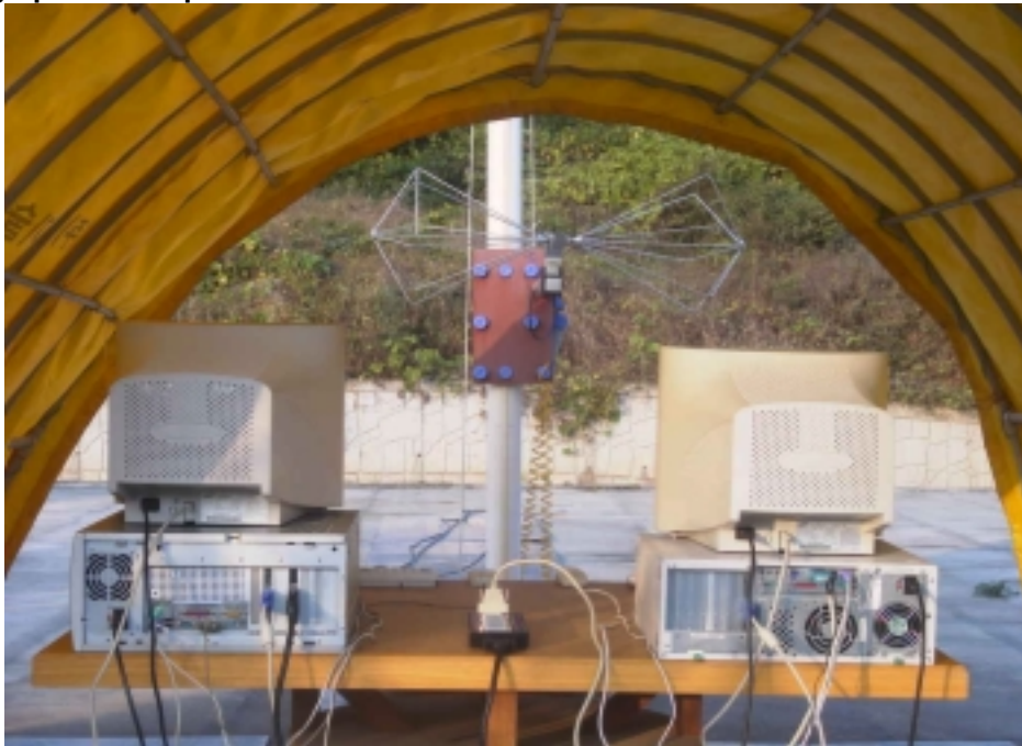
Photograph 1 : Setup for radiated Emissions
