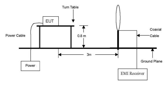
The diagram below shows the test setup that is utilized to make the measurements for emission from 30 Mb to 1 Gb Emissions.
