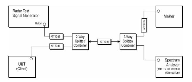
The radar signal generation equipment consists of a vector signal generator
