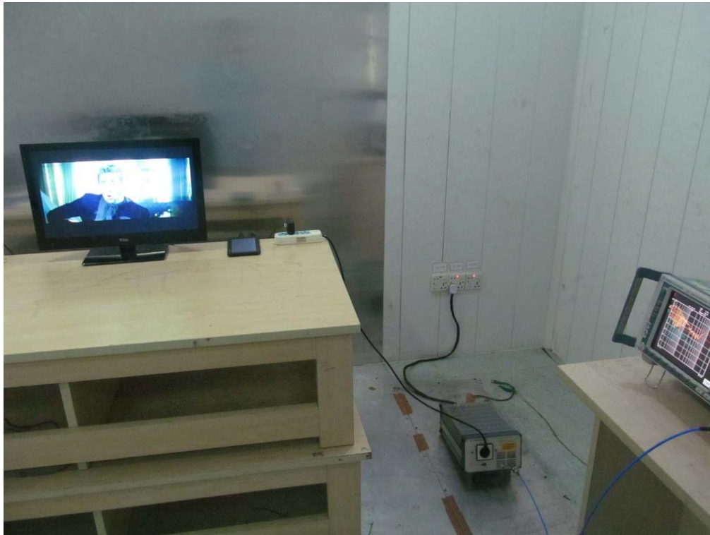
FCC RADIATED EMISSION TEST SETUP
