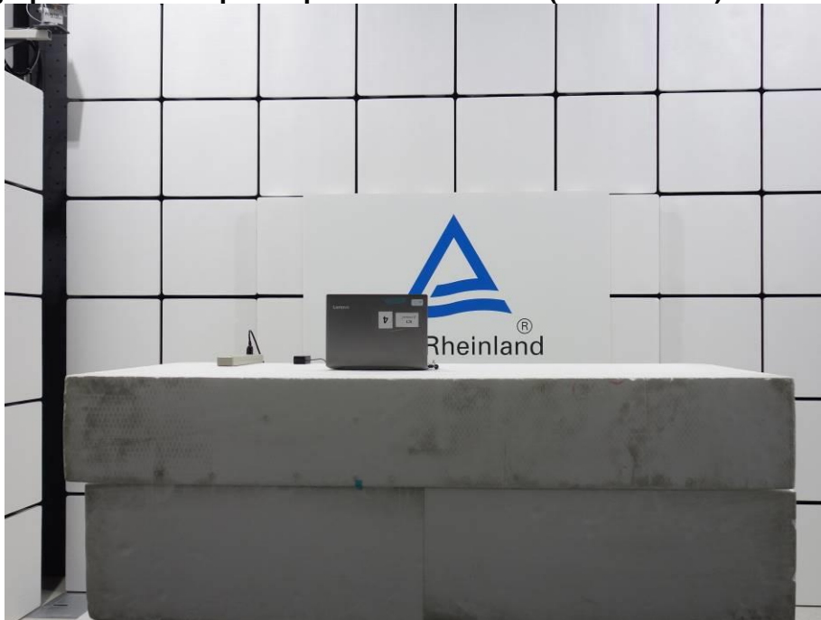
Photograph 2: Test Setup for Spurious Emissions (Front View 2)
