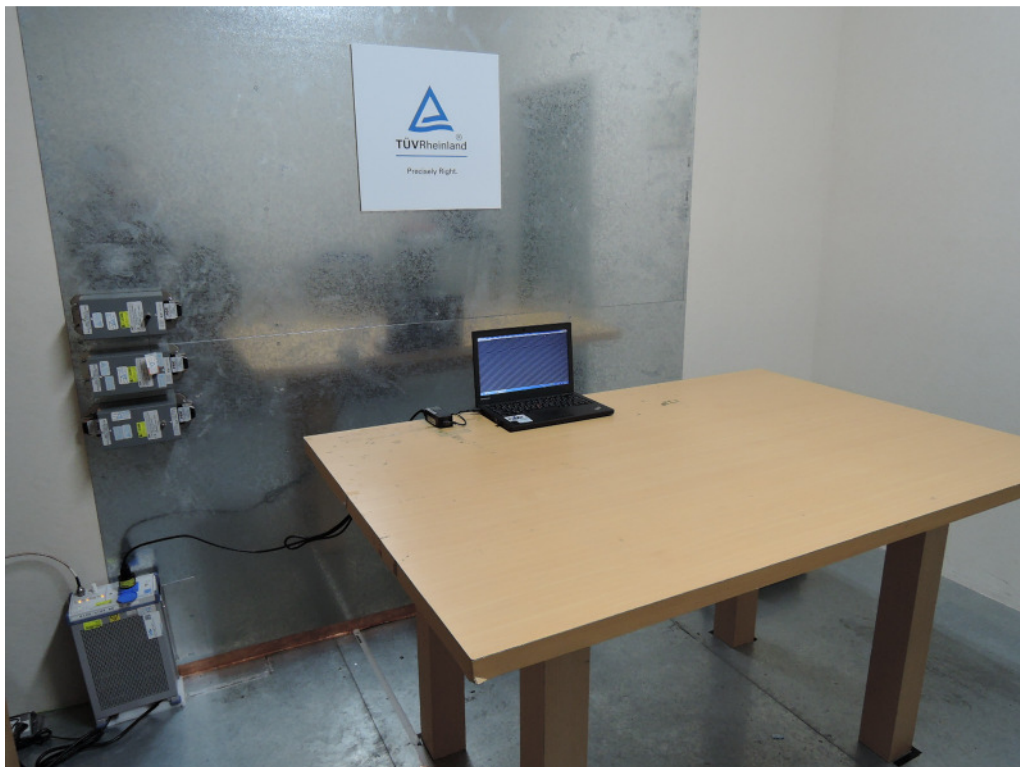
Photograph 6: Set-up for for Mains Conducted testing Front
