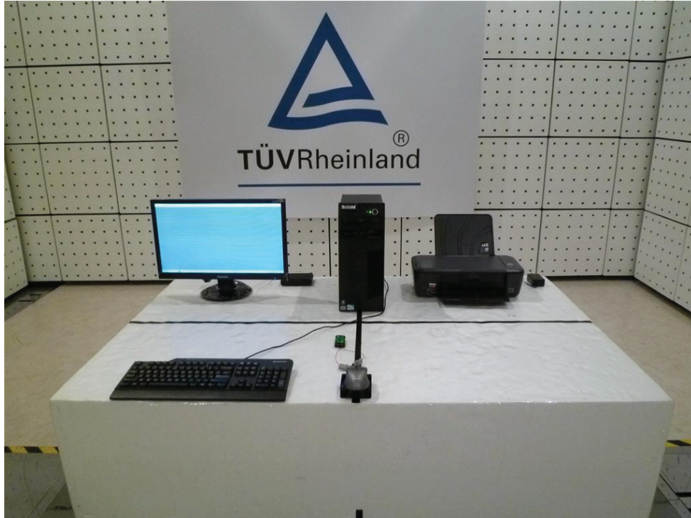
Picture 2: Radiated Emission, 30 - 1000 MHz
