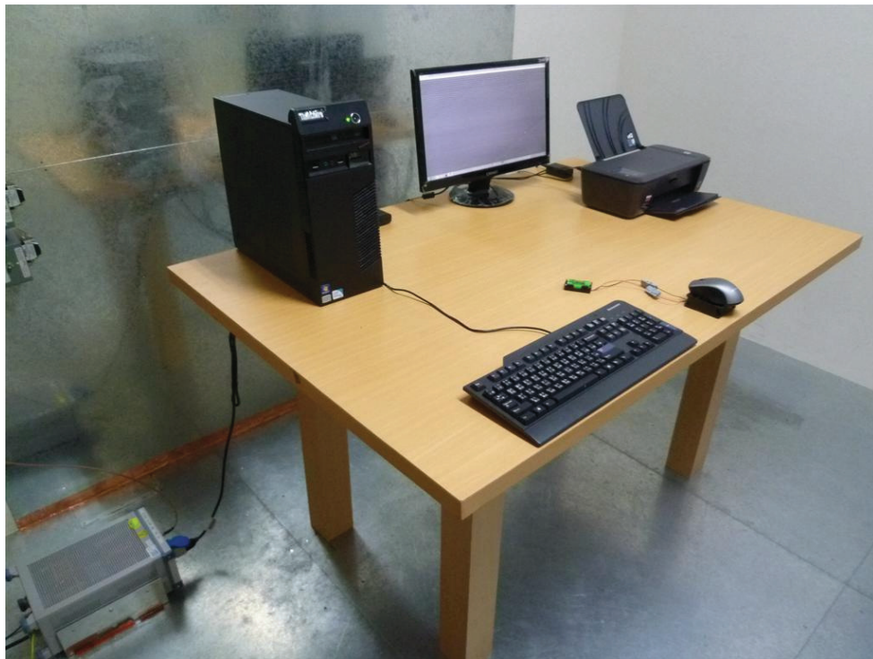
Picture 1: Conducted Emission, AC Mains; 0.15 – 30 MHz
