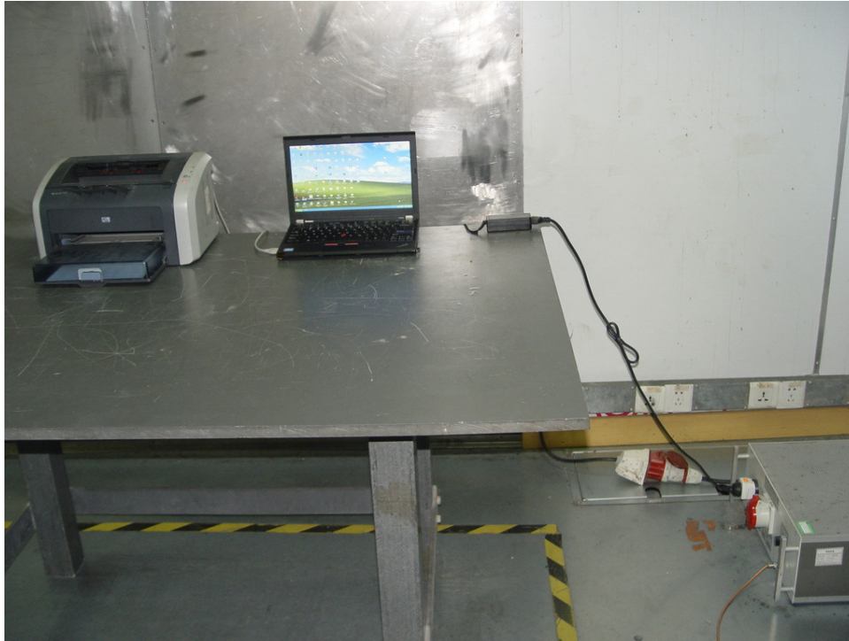
Photograph 5: Set-up for Conducted Emissions
